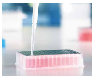
50 – 1000 µl pipette tips in a deep-well plate
